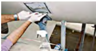
Vådslib for at fjerne gammel bundmaling
