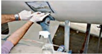
Wet scrape to remove old antifouling
