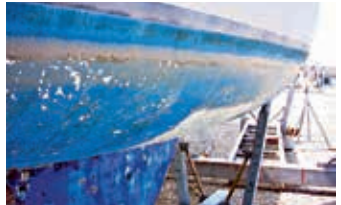
Paint blisters and lifts
