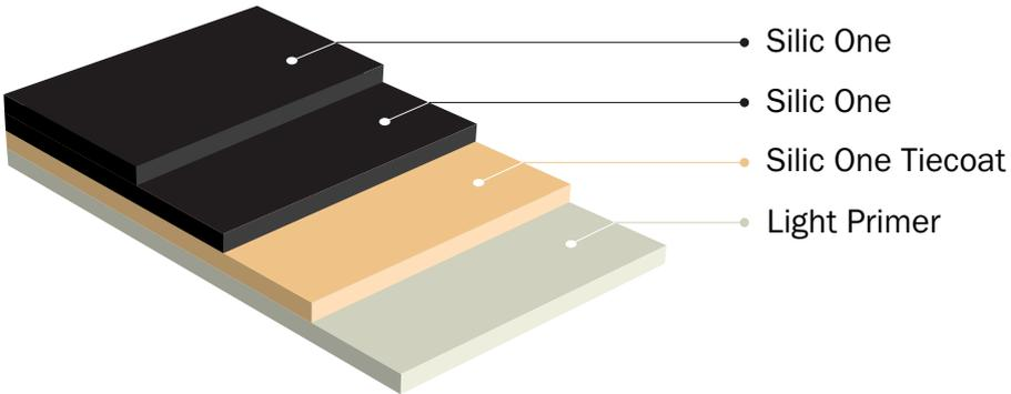
Note: New gelcoats need to be epoxy primed to a minimum of 300 micron dry film thickness.
