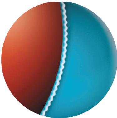
Unique, non-reactive polymers form a hydrogel layer between the substrate and water.
