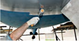
Aplicar Hempel's High Protect II a rodillo
